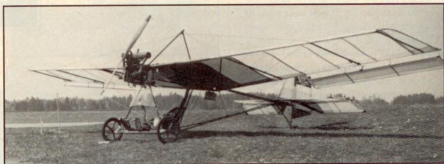
Today's ultralights, represented by the Robertson B1-RD (above), are improvements on the Demoiselle. Reduction-drive gearing, conventional pilot controls and tail surfaces and ailerons for lateral control are some of the B1-RD's innovations.
